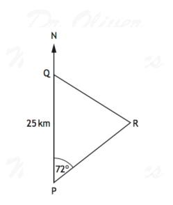
Portlee is 25 kilometres due South of Queenstown. From Portlee, the bearing of Rushton is  $072^{\circ}$ . From Queenstown, the bearing of Rushton is 128°.
