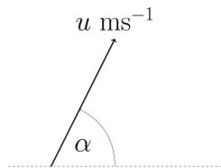
In the absence of air resistance, the horizontal component of the velocity,  $u \cos \alpha$  will remain constant; the the initial vertical component of the velocity,  $u \sin \alpha$  will change across time (just as in *Mechanics 1*) due to the influence of gravity.
